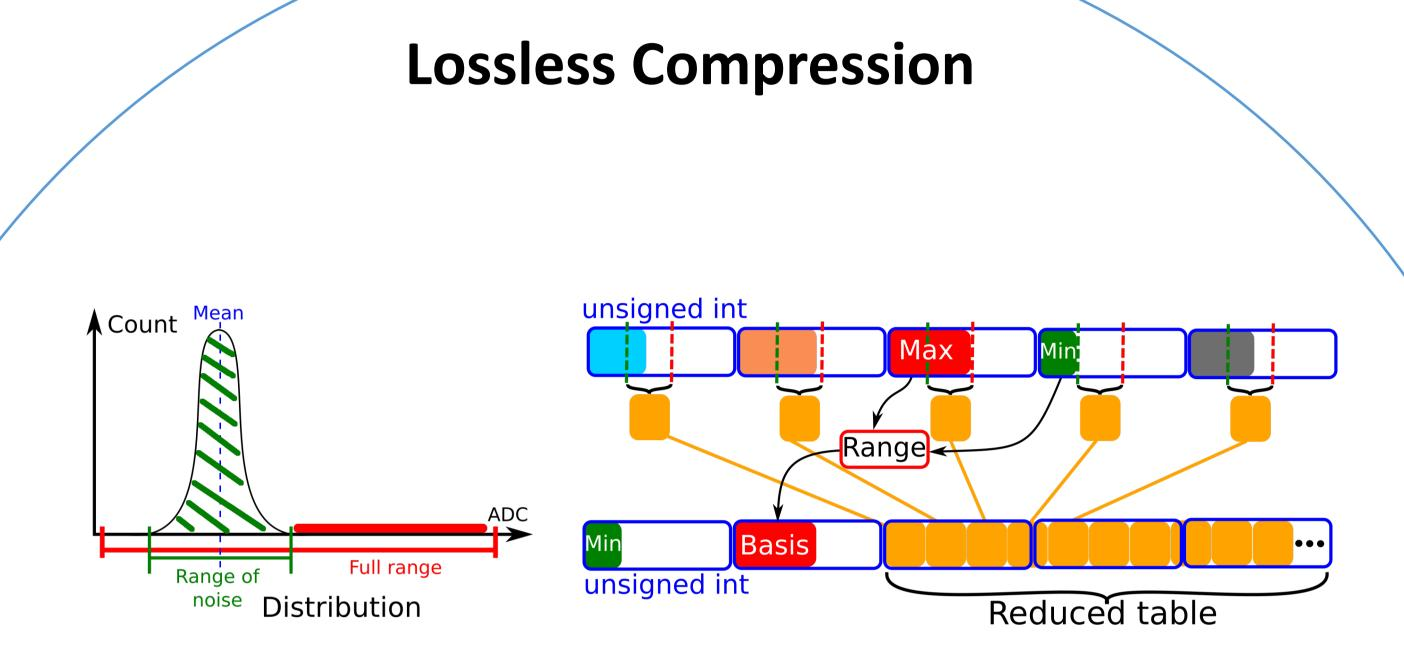
Physics digitalized signals consist of integers. But the signal range (basis) is usually much smaller than the range of the values storable in an unsigned int. Knowing the min value and the basis of the signal, it can be stored as a single chunk of binary data (reduced table).
