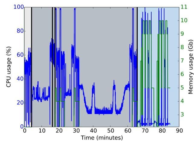
Complementary to the timings in the diagram, the WFC can be used to characterise the resource utilisation at run time. Here it is shown at what time the bottle necks occur, and whether the system is fully being efficiently utilised. Together, such plots can be used to decide on what parts of the pipeline to focus R&D efforts.
