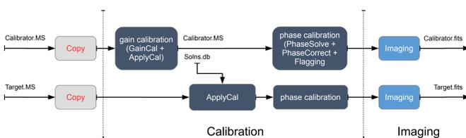
Graphical representation of the pipeline used for this demo. The pipeline consists of generating an image based on a target and calibrator observation. For this demonstration, we execute on a single LOFAR subband, averaged by a factor 32. The colours in the image match the colours in the results shown later.
