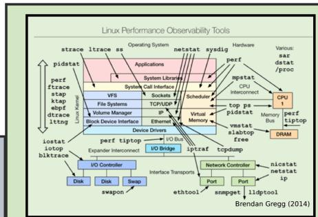
As can be seen in the image, the Linux kernel provides many probe points for system resource monitoring and application characterisation. The multitude of probes, tools and methods of which each has their own complexity when interacting with the system, makes it hard to obtain numbers that are reproducible with different hardware and software.
