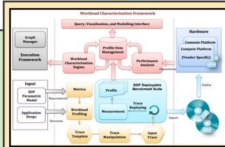
The Workload Characterisation Framework (WFC) is developed as part of the SKA Science DataProcessor (SDP) element. The goal of this framework is to support future operations, planning and R&D efforts. The Figure above shows the components from which the WFC will consist. It aims to provide a uniform method to characterise workloads in atlescope, with provenance making it suited for other use cases as well.
