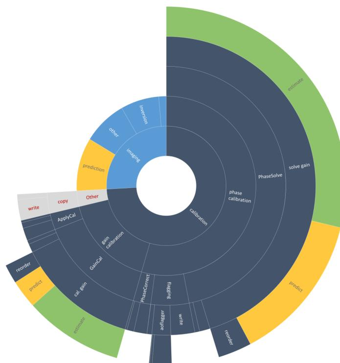
A hierarchical overview of the timings obtained by characterising the pipeline. The most time consuming steps — predict and estimate — are emphasised.
